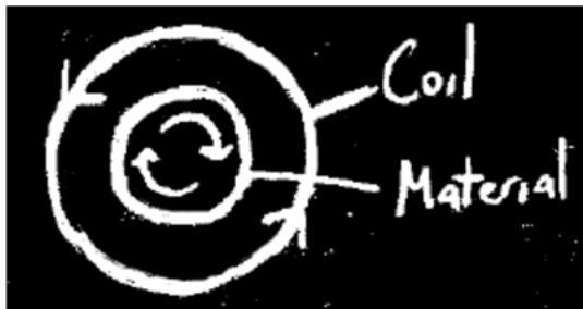
Fig 4: Eddy Currents Caused By Induction
