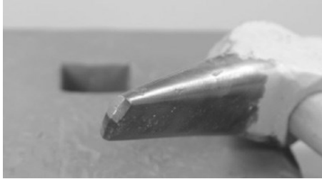
The hammer-eye punch has a slight point and is bevelled on each side. Punch is 1/2" wide by 3/16" thick
