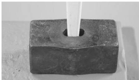
Support the block over the hardy hole and drive in the tapered drift
