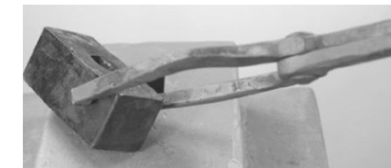
The bar should continue to pivot between the jaws as you continue to turn the tongs
