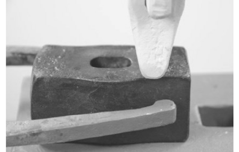
'Being flat, the stock will sit on the anvil as you create a fullered groove defining the body and the faces
