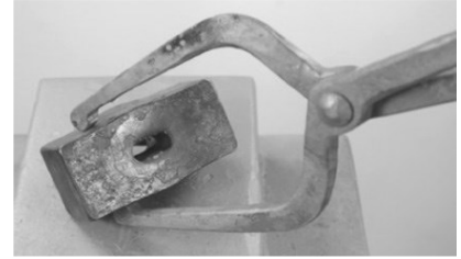
To turn the bar end-for-end, lift the tongs and turn the bar to lay on its left corner
