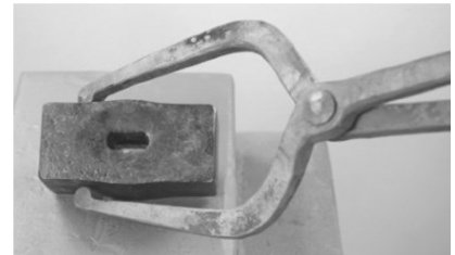
Continue to turn the tongs to the left (counterclockwise) allowing the bar to pivot in the tongs
