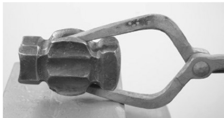
Tongs gripping the stock with the tips of the jaws in the hammer eye
