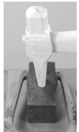
Turn the bar over and punch from the other side, again turning the bar end-for-end as you work
