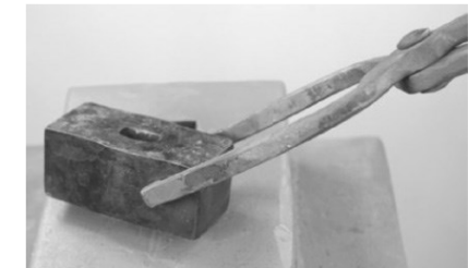
The bar should continue to pivot between the jaws as you continue to turn the tongs
