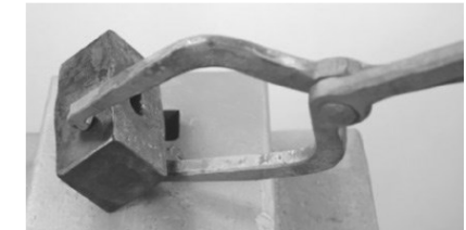
Continue turning the tongs to the left. Note the jaws of the tongs are drawn for support where they make a bend
