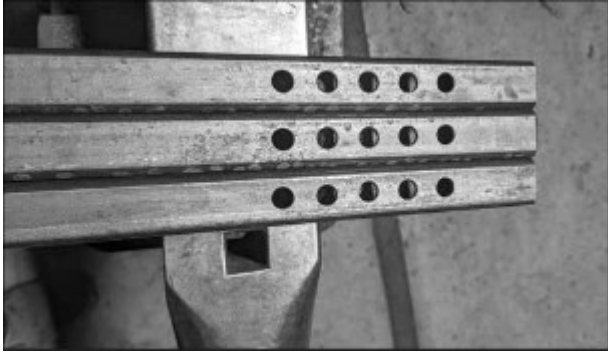
Drill all the holes and remove any swarf
