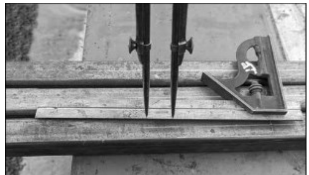
Use dividers to mark out the adjustment holes. Mine are 1 \frac{3}{16} " on-center
