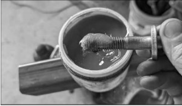
Dip the threads of the bolt in anti-spatter dip before assembling the bolt through the leg and positioning the nut
