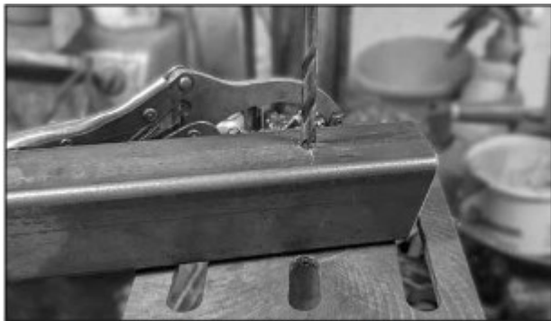
The retaining bolt is 2" up from the bottom of the outside leg on the straight cut side
