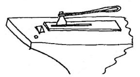
of 1" wide stock. The chisel or hot cut should have a rounded end so it can be rocked along and kept in the same groove. Grady used a handle made of 1/4" round stock wrapped around the chisel so that it could be requenched and tempered easily.
