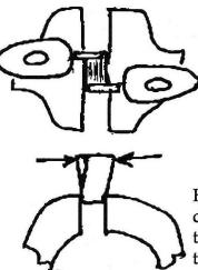
tom of the collar in a vise and bend the ends to straighten. It will still be twisted but you can hammer it straight while closing it.
