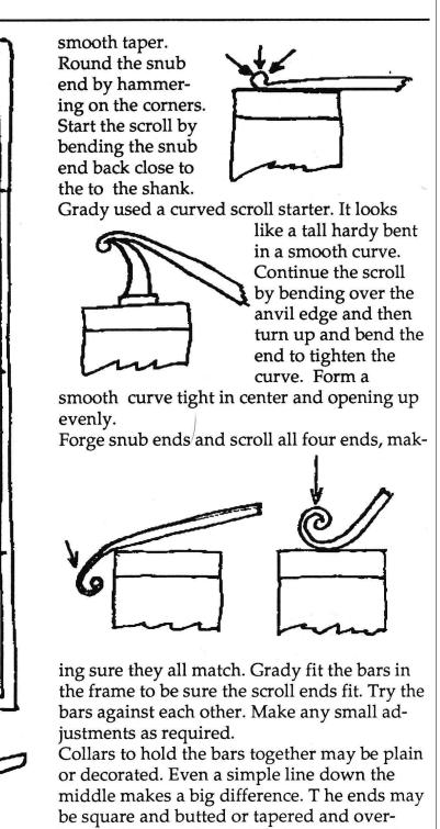
lapped. The length of collar is perimeter of bars + 2 1/2 times the thickness of the collar stock. This is true for either tapered or butted ends. ©Clay Spencer1991
