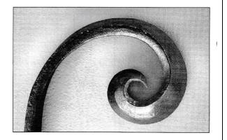
Getting to the very end of the scroll can be difficult. In order to get to the end, you will have to knock the end out of alignment. Take **Step 2E** and finish scrolling, using your hand hammer on the face of the anvil.
