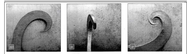
When you bevel the inside edge, the scroll will open; when you bevel the outside edge, it will close the scroll, making it tighter.
